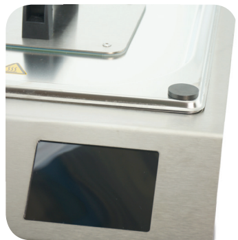
Figure 2. The lid needs to be oriented in such a way that the magnet is on the corner closest to the display.
